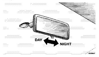
Annoying headlight glare can be reduced by moving the small control under the mirror to the night position (toward rear of truck). The mirror should be adjusted while set in the day position (toward windshield).
